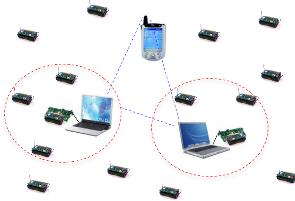
Fig. 2. Operational scenario showing one hop communication between base stations (laptops) and sensors and multi-hop communication among base stations and clients (PDAs). Client agents can also be co-located with the base stations (e.g., running on the laptops).
